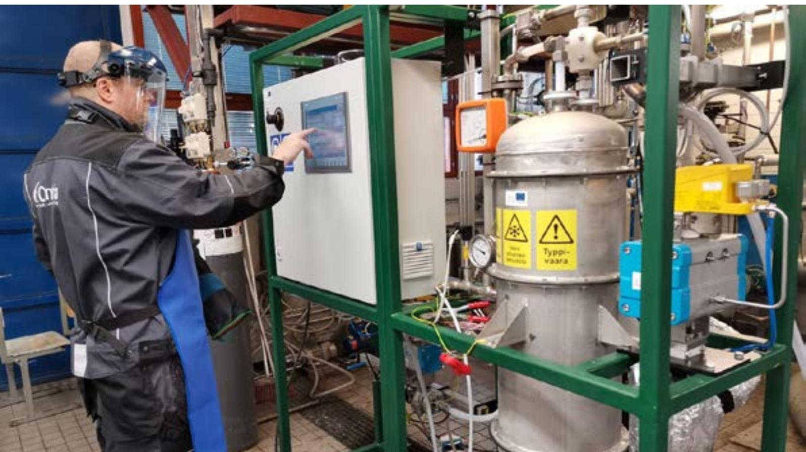
The aim of the project is to develop a new technology that will enable the small-scale liquefaction of biomethane in a cost-effective way. The liquefaction solution is based on the principle of cryogenic processing, which utilizes very low temperatures instead of high pressures to condense the gas.
